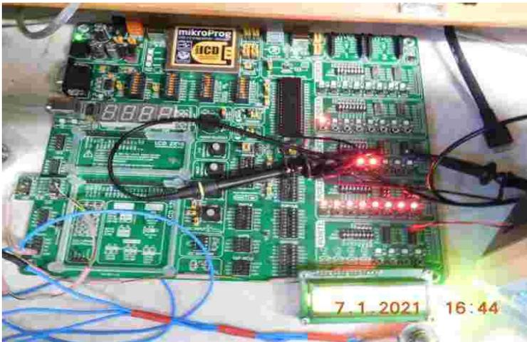
The compiler was based on MIKRO C compiler and the EASYPIC Version 7 development board. This enabled the code to be written and debugged using the minimum of hardware. When the meter was built an off board debugging used to refine the code in conjunction with the real hardware in real time.
