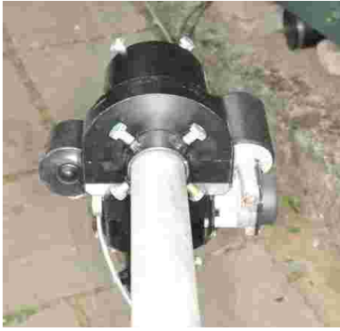
Figure 1: SPID rotator showing AZ and EL motors
